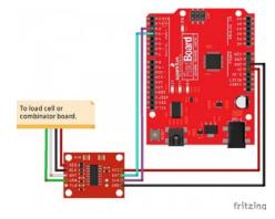
Fritzing diagram of HX711 amplifier connected to a RedBoard
