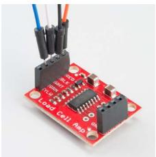
Load cell wires hooked up to the HX711 Amplifier board
