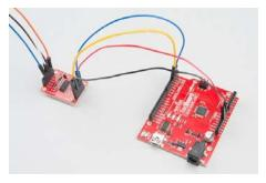
HX711 Amplifier board hooked up to a RedBoard
