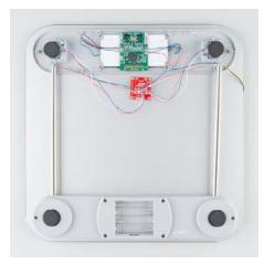
Hacked home scale's four load sensors hooked up to our combinator board
