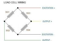
Four strain gauges (SG1 through 4) hooked up in a wheatstone bridge formation
