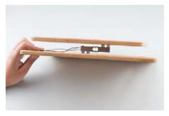
Bar load cell between a two plate configuration
