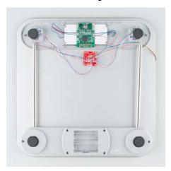
Possible four disc load cell configuration in something like a bathroom scale
