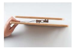
Note that only one side of the load cell is screwed into each board. This provides a moment of force, or torque, on the strain gauge rather than just compression force, which is easier to measure and much more accurate.
