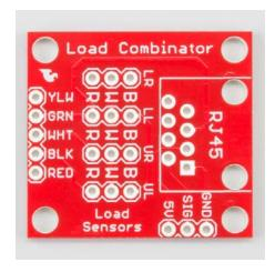
The combinator board also has room for an 8 pin RJ45 socket, which can be used to connect your project via Ethernet cables for long distance applications.
